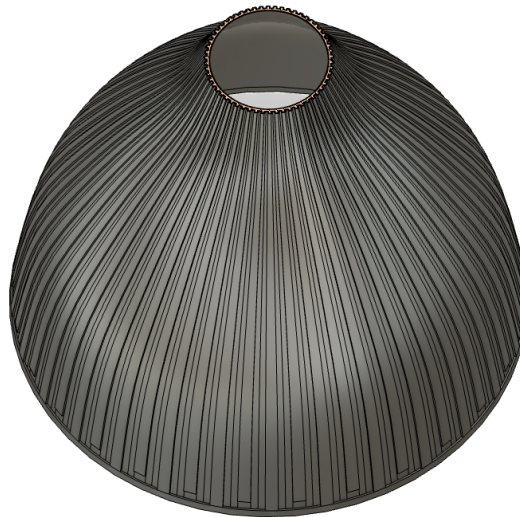
Figure 8: Regenerative cooling channel design
