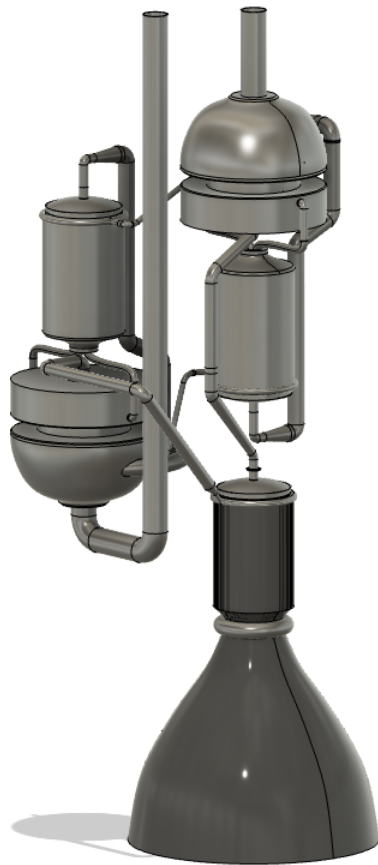
Figure 1: HyperX 3D rendering image. For better visibility, no structural support is added, and components might look bigger in size than the actual geometry or showcase larger space between components
